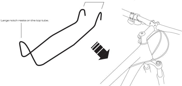
Two hooks hold on to the handle bar to the left and right of the stem.
