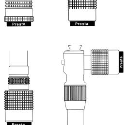
Depending on the model, Birzman pumps are equipped with either a straight or L-shaped Snap-It Apogee valve head.
